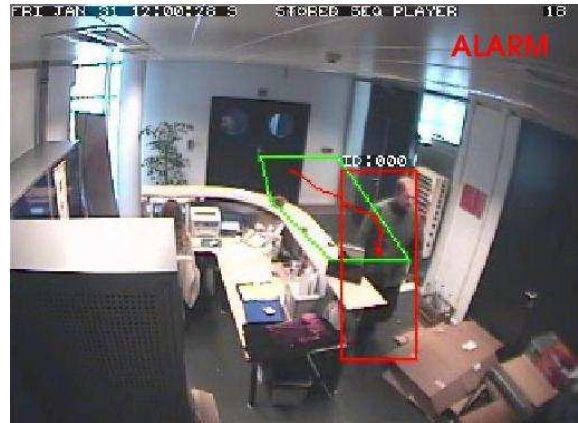
Figure 3 : Alarm generation for a human intrusion in a predefined area of interest.
