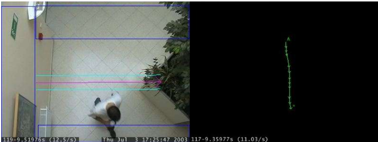
Fig. 8. Display of people counting module. Left: video and context, right: tracking result.
