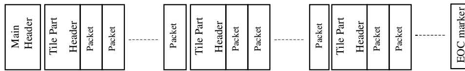
Figure 4: JPEG 2000 codestream structure
