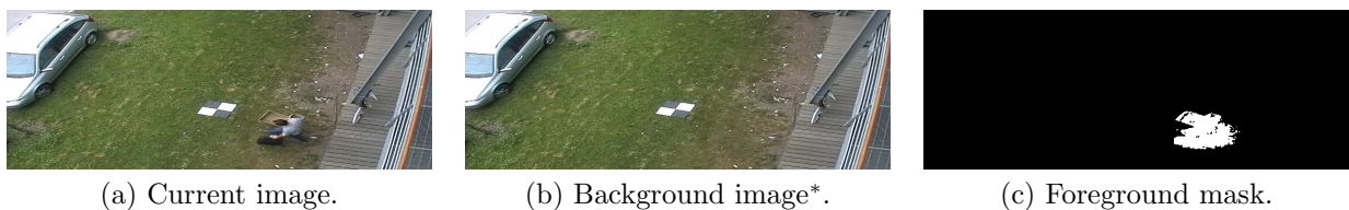
Figure 2. Moving object detection results obtained through Gaussian Mixture Model.
