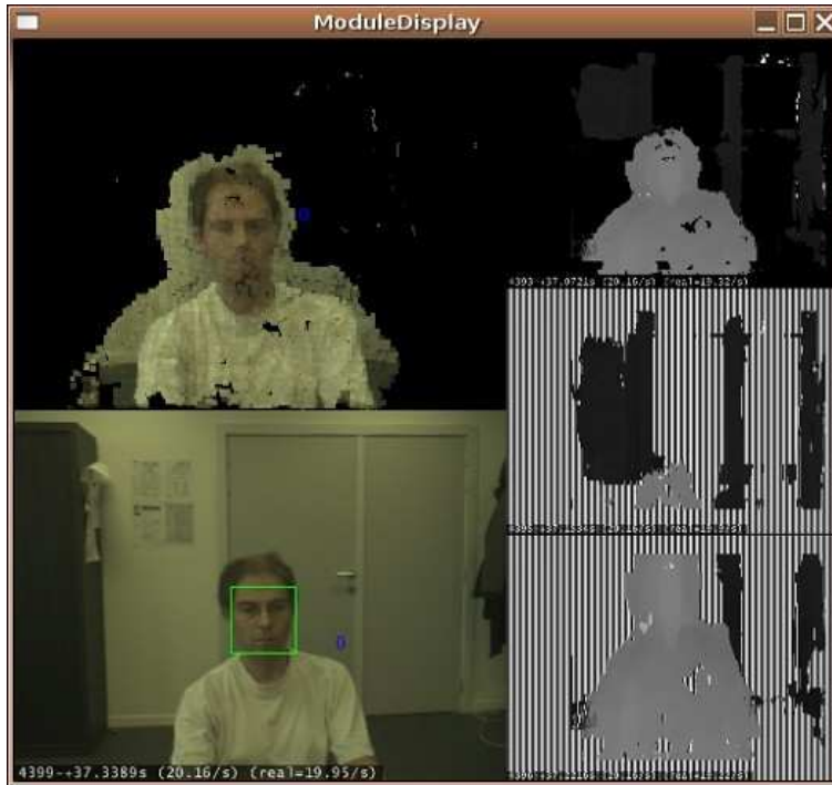
Figure 2. Validation display of the CS. Top left is the 20K point cloud of the user. Bottom left shows the detected face (green rectangle). Upper right is the depth map. The two small images on bottom and middle right are the results of the parallel computation of the upper and lower parts of the depth map, which are then superimposed to form the complete depth map (upper right).
