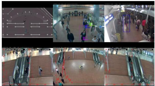
*Situational reporting tool – aiming at reporting passengers location (cf. dots at escalators and in the hall, tracks on footbridge) on the infrastructure ma.*
