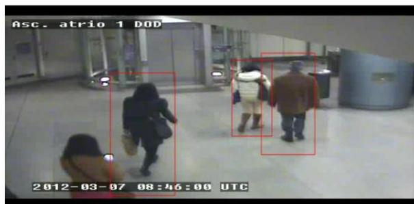
*Human detector – allowing to detect passenger's presence in the data stream.*
